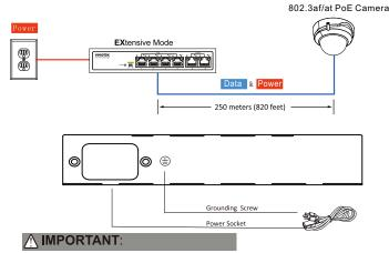
The switch already comes with lightning protection mechanism. You should always ground the switch through the PE (Protecting Earth) cable of AC cord or with ground cable. Not grounding the power may cause the power input to damage the unit.
